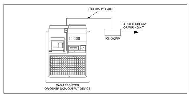
Figure 2. Interface Cable Connected to Data Output Device
